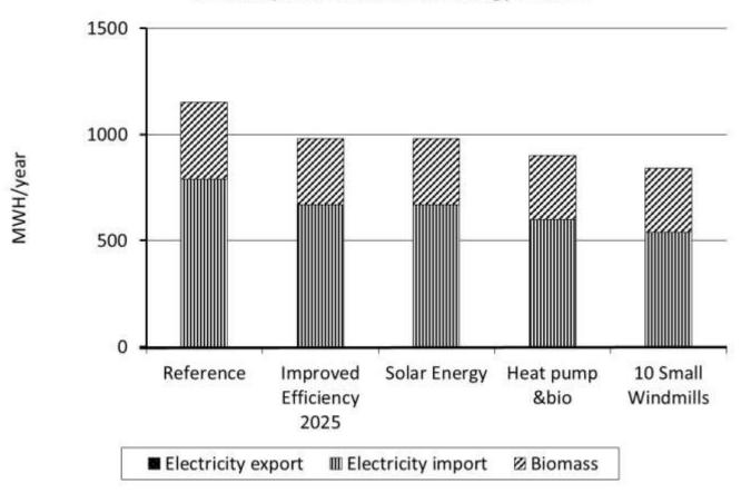
Wind power is only shown with small windmills (Otherwise the scale would make it difficult to read the differences up to the installation of windmills). We see that the effect of the big windmill is a combination of less consumption from and export to the net.
