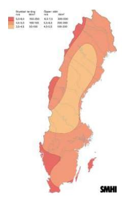
The wind energy with measurements in 50 m heights, Source SMHI, lies about 4.5 - 5,0 m/s and 100-150 W/m2 in sheltered areas and 5.5-6,5 and 200-300 W/m2 in more open areas.
