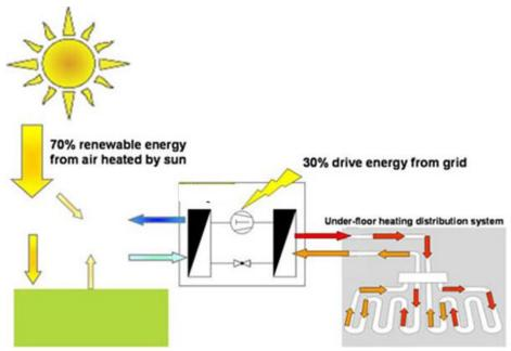
Figure 1 Air to Water heat pump for Eivers Lane Childcare
