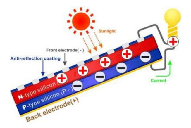
Light consists of packets of energy called photons. Depending on their wavelength, photons are either reflected or absorbed. The energy from the absorbed photons is given to the electrons in the material, which causes some of them to cross the p-n junction. Both cell sides must be connected in order to get a current flow. Current is proportional to the number of absorbed photons and therefore proportional to the light intensity.
