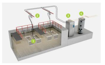
Waste Water Heat Pump System (Evertech), design chosen for Kittelfjäll pilot site
